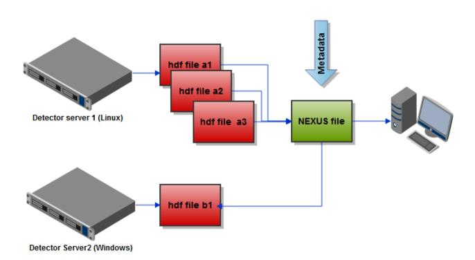
Figure 1 gives a schematic representation of an experimental setup found increasing frequently where multiple detectors are configured for one experimental procedure. In the case of high data rate or complex experiments data may originate from a number of detectors and practically is stored in separate files written directly by the detector server. The consistency of the NEXUS file is implemented using the NXDataFile constructor together with the associated metadata.
