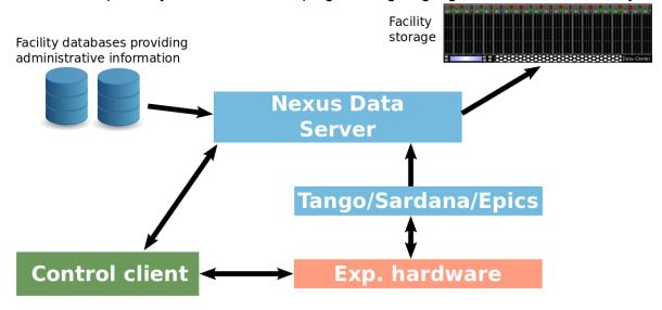
We thus have decided to move the responsibility for data IO out of the control client (CC) into a separate Tango server: the Nexus Data Server (NexDaTaS). To communicate with this server the
