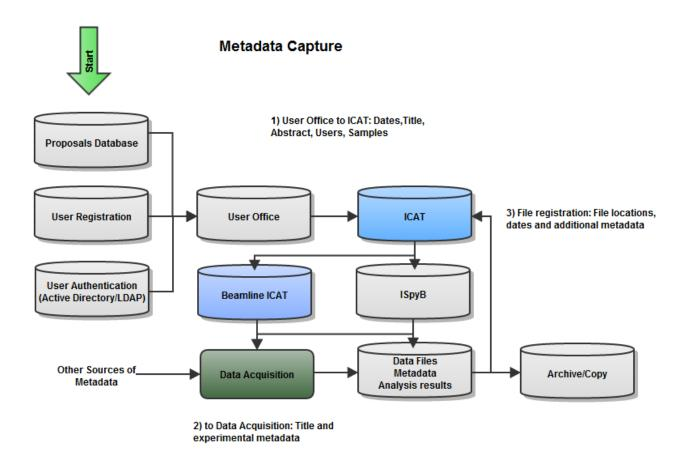
Figure 2 – A schematic view of the association of metadata to acquired data at the Diamond Light Source. This is analogous to the systems currently available at other facilities. The overall aims of PANData should provide the necessary software and infrastructure to implement this elsewhere.
