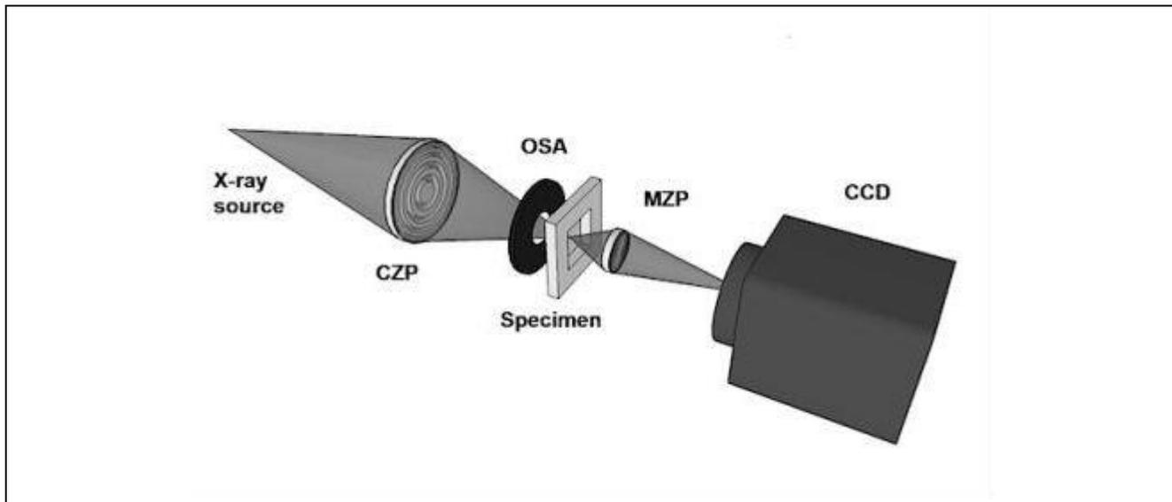
Figure 6: Outline of Full-field imaging setup in TwinMic
