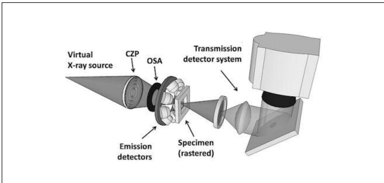
Figure 7: Outline of scanning X-ray microscopy setup in TwinMic
