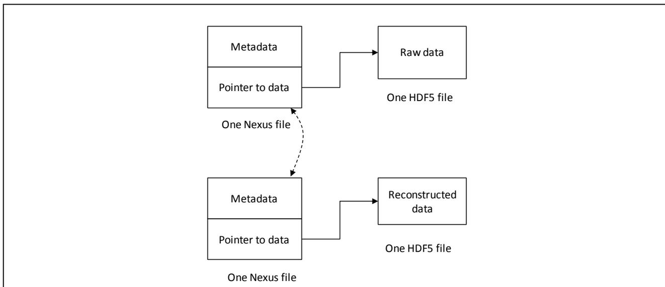
Figure 17: The Relationships between the metadata file and the data file.
