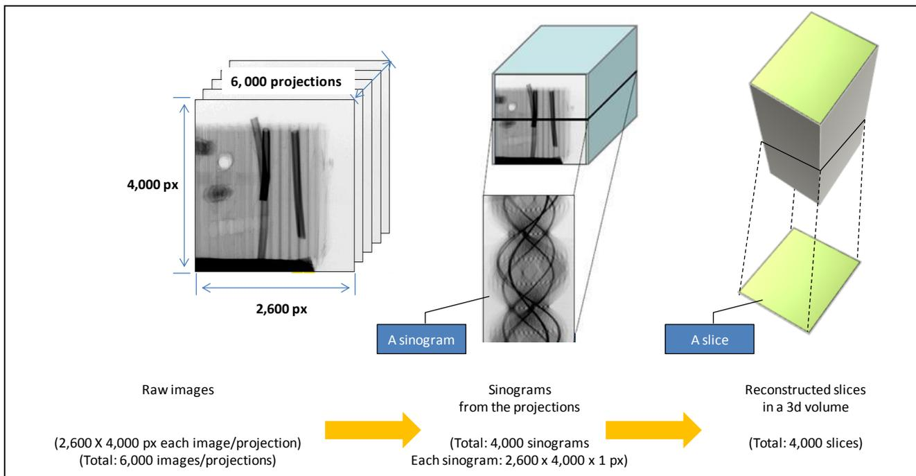
Figure 16 : Sinogram Generation and Image Slice Reconstruction (Part Image Courtesy: Dr. Mark Basham, Diamond)
